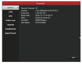
Note: The status of "Nat Status" on this page will only be displayed as "Connected" once the network cable is connected to a properly connected router and the IP address is configured in the network settings of the XVR.
